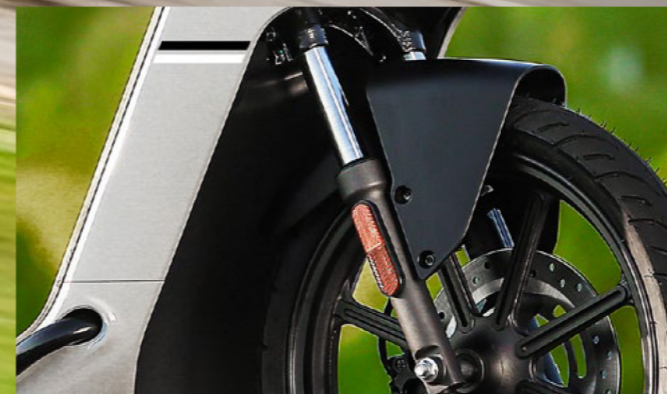
Front suspension diameter \varnothing 31mm
