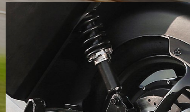
Rear suspension diameter \varnothing 32mm
